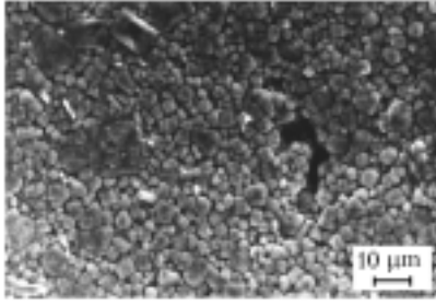
Fig. 1. Photograph of the microstructure of posistor ceramics.
